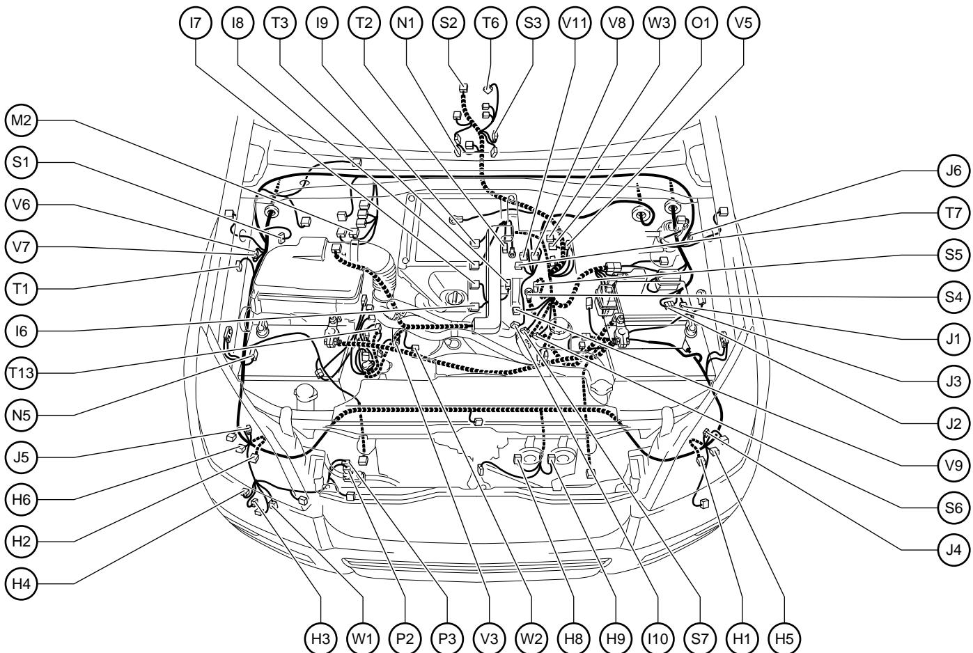
H 1 Headlight Beam Level Control Actuator LH
