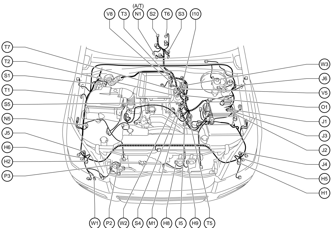
H 1 Headlight Beam Level Control Actuator LH
